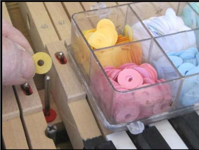
Once the measurement has been made for the key, leveling papers are added at the balance rail to bring the height of the key up to level. Papers as thin as .001" are used to produce a perfectly level set of keys. After all the keys have been leveled, the leveling papers and the balance rail felts will be flipped so that the felts are on top.
