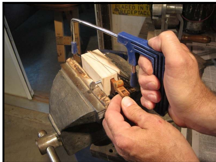
Special sawing jig required.
