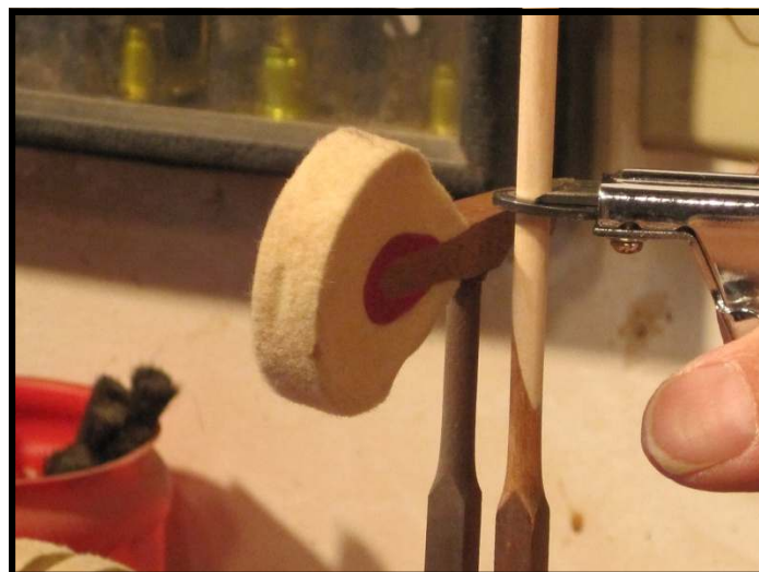
Newly spiced shank being cut to length.
