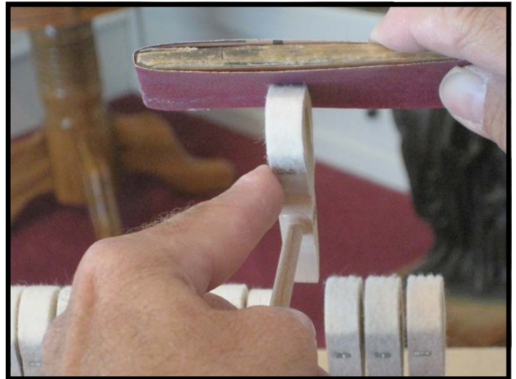
Hammers being filed to remove cut marks.
