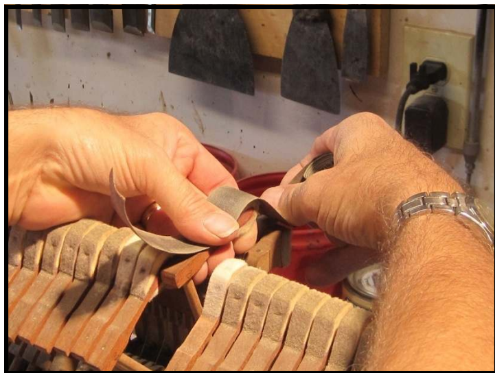
Hammers being filed to remove cut marks.
