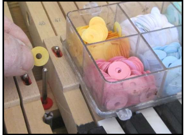
.03" inch paper punching being installed
