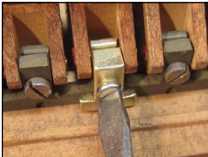
Repair clip for broken tongue being installed.
